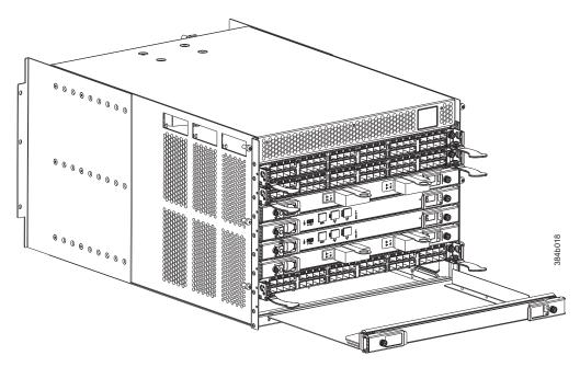
Figure 34. Filler panel removal and installation
